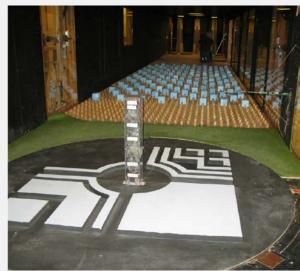
Wind loads measured in a wind tunnel experiment will be used as input data, to study the effect of different heights of the high-rise building.
